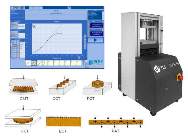
The Testing Software allows to perform Compression tests on standard samples of corrugated paper and cardboard such as: CMT - RCT - ECT - FCT - PAT
