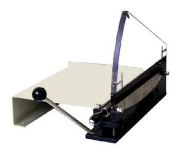
Before cutting, press the lever which meets the fixed cutter blade at the guide end. This clamps and thightens the sample and therefore ensures that high accuracy is obtained.
