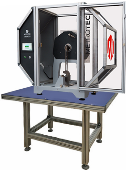
Impact Test Pendulum PIT-25 + table Support (compliance to standards >15Joules)
