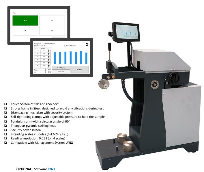
Through a PC and LYNX Single Software + Puncture Test Module, it is possible capture quickly and reliable results of the tests. Later it is possible to make statistical calculations
