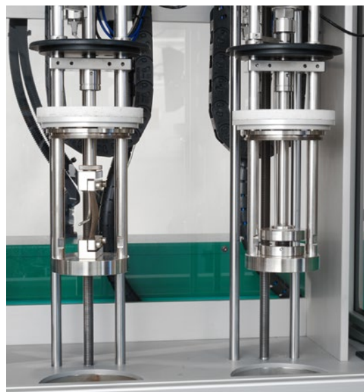
Test station for testing in compression and for testing in tension.
