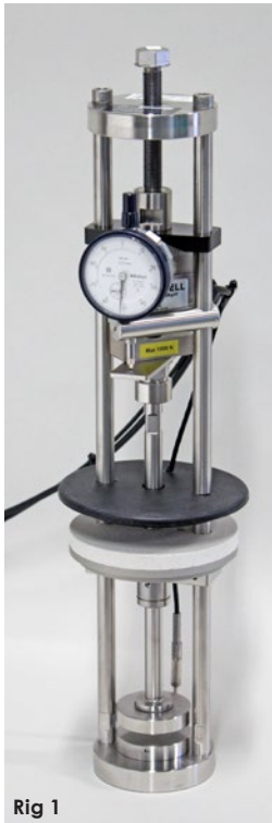
Rig 1 is arranged for testing in compression according to ISO 3384.
