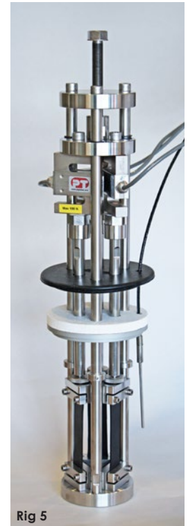
Rig 5 is a triple rig where you can perform a triple test in the same rig.
