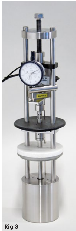
Rig 3 is arranged for testing in liquid according to ISO 3384.
