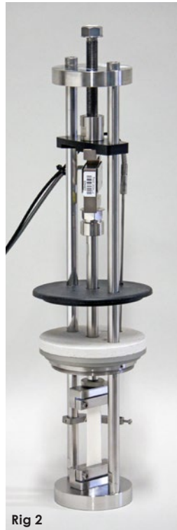
Rig 2 is arranged for testing in tension according to ISO 6914 method A.
