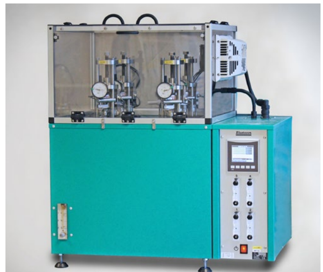
Cell oven EB 21LTHTP for relaxation tests with 4 cells with individual temperature control and cycling between RT to elevated temperature.
