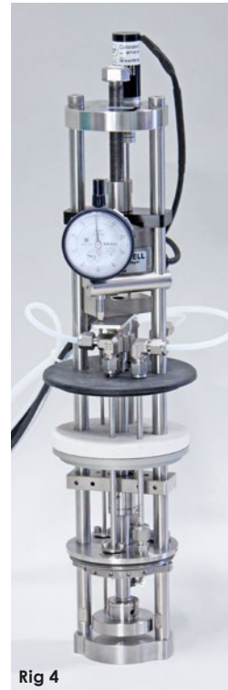
Rig 4 is arranged for testing according to ALE-test.
