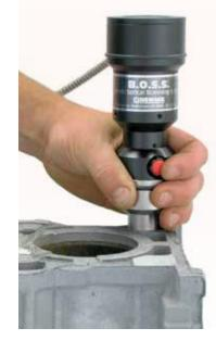
of the impression. Using the image to accurately measure the diameter, the system displays the resulting Brinell value, the diameter measurement, and the identified edges at 8 positions.
