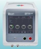
**Uson's Sprint**<sup>mD</sup>—A flexible solution for leak testing a wide range of components using the pressure decay method.
