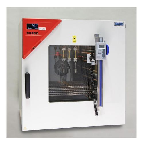
**The EB 30 hot set oven basic** is made for hot set testing of cable material according to IEC 60811-507 and technically equivalent standards.
